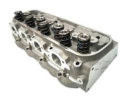
**Head Gaskets:** When using BMP BBC 16 Degree heads on Mark IV blocks use the corresponding gasket that is compatible with the bore size of the engine.4.370" = Felpro 1027, 4.540" = Felpro 1017 & 4.630"= Felpro 1057. When using a BMP BBC 16 Degree head on a Mark V or VI block, you must use Mark V or VI head gasket depending on which one was used
