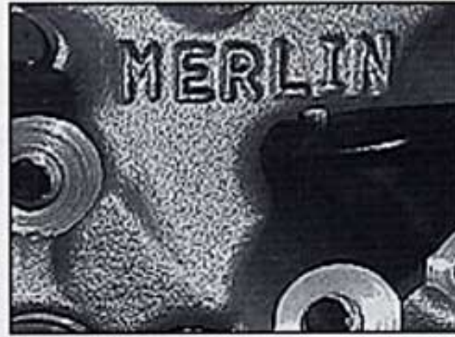
The name Merlin™ is cast on top of the heat crossover area. TIP: An easy way to tell a World casting from its competitor is to look for a heat crossover. Other brands have deleted this boss.
