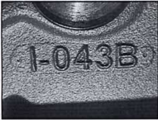
"I-043" is cast below the left-most intake spring pocket. The letter (B, C, D) designates port size/shape. I-043B: 345cc rect port, I-043C: 310cc rect port, I-043D: 269cc oval port.
