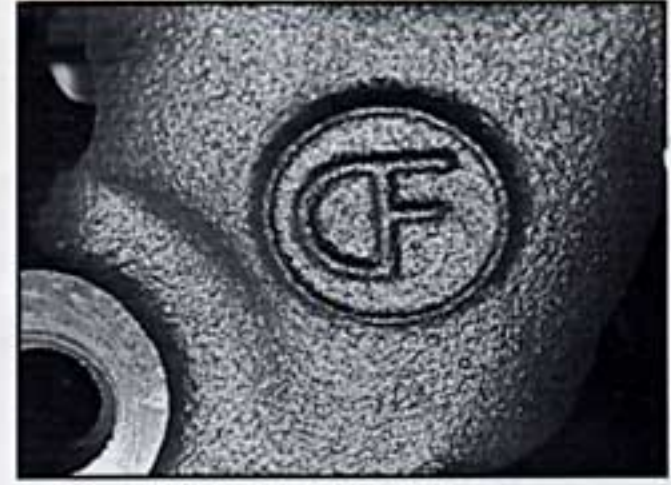
As with all World Products castings, the foundry mark is easily identified. On the Merlin™ the mark is cast on the left-most intake runner. Different foundries have been used through the years.
